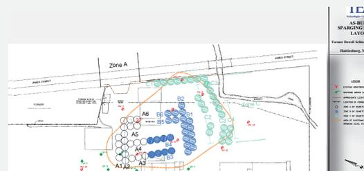
The system includes a forced air system with air compressors, an air distribution system, and air sparging wells located throughout the site. The system layout includes a total of 71 sparging points within three zones, designed to balance the air flow to each zone.
